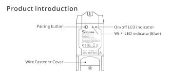
(1) The device weight is less than 1 kg. The installation height of less than 2 m is recommended.
